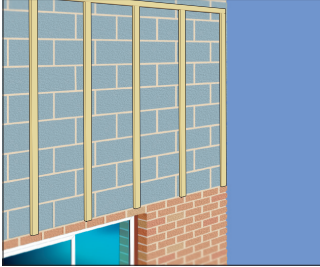
1. Fix perimeter frame and intermediate vertical battens to wall
